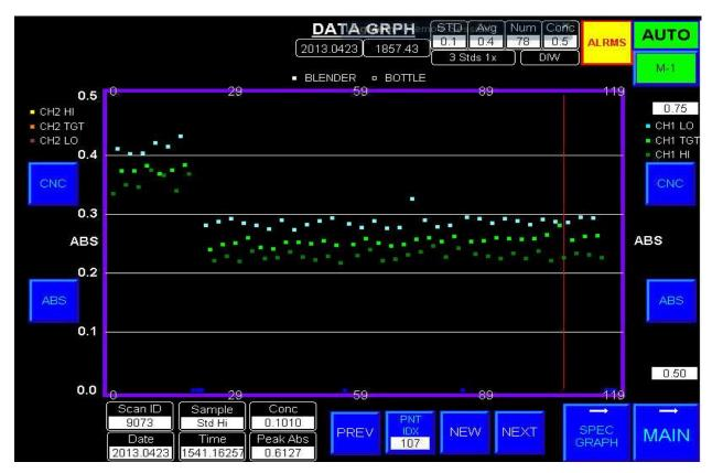
The system is available as either a process instrument designed for 24/7 automated process monitoring and control, or as a bench-top instrument. The sample results can be reported via an Ethernet/IP (Allen Bradley Compact Logix PLC), a hardware interface (4-20mA / Dry Contact), or local printer.
